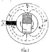
Fig.1 shows a device that uses permanent magnets as the rotor. The magnetic flux is concentrated in ferromagnetic ring. The structure of this field consists of two parts. The direction of flux in one part is opposite to the direction of flux in the other part.
